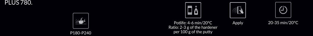
3. Sand down the defects (scratches or dents) with P180 to 240 sandpaper. Blow away all dust and degrease with PLUS 780.
