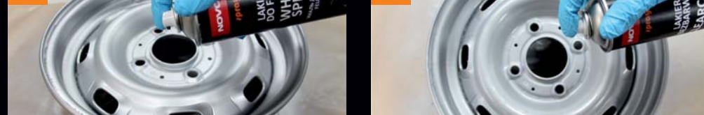
6. Apply the ACRYLIC PRIMER to the area of repair. Sand down with P400 to P500 (dry) or P800 to P1000 (wet) sandpaper. Blow away all dust and degrease with PLUS 780.
