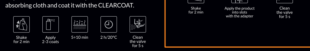
9A. Wipe the cured basecoat layer clean with the dust-absorbing cloth and coat it with the CLEARCOAT.
