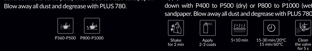
5. Sand down the cured putty with P280 to P320 sandpaper. Blow away all dust and degrease with PLUS 780.
