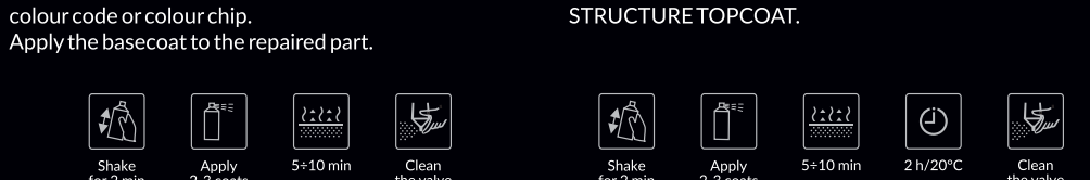
8B. If you want to reproduce the texture of plastic, apply the STRUCTURE TOPCOAT.
