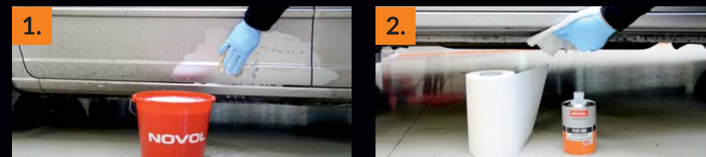
1. Thoroughly wash the surface to be repaired with water and a detergent.
