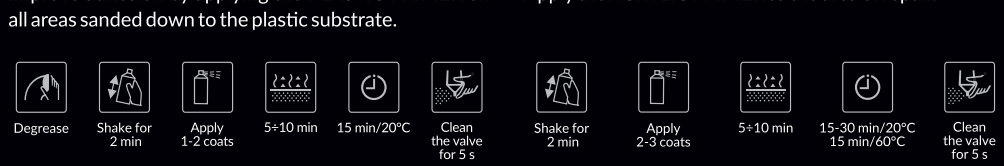
5. Improve adhesion by applying the PLASTIC PRIMER on all areas sanded down to the plastic substrate.
