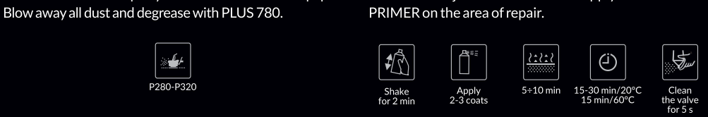
5. Sand down the cured putty with P180 to P320 sandpaper. Blow away all dust and degrease with PLUS 780.
